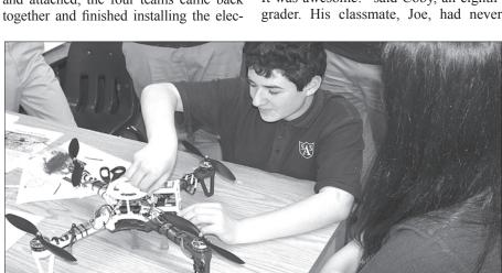
A student helps assemble the quadcopter, which gets its name from its four helicopter-like propellers mounted on arms extending outward from a central body. The project began with the printing of the quadcopter's frame on the school's own 3D printer.
